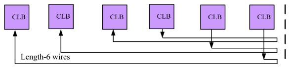
Mux + Buffer architecture as routing switchesc
