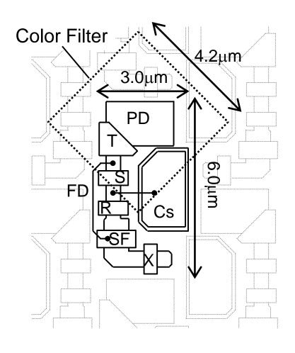
Rectangle Pixel Structure: High Area Efficiency Large Size PD: High Sensitivity
