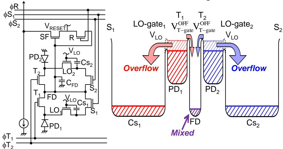
**Sharing Pixel Components: High Resolution LOFIC Technology: High Full Well Capacity**
