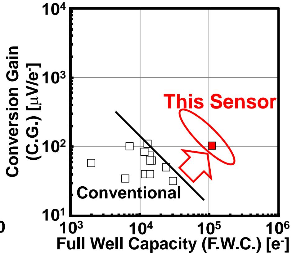
A low noise and high F.W.C. CMOS image sensor has been developed by using column source follower readout circuits.
