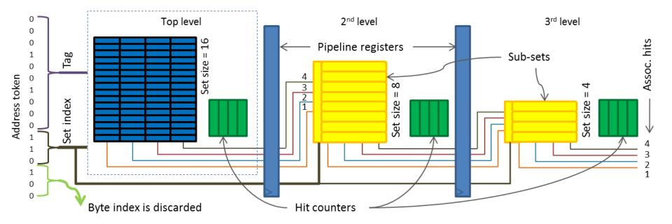
Enables the simulation of caches of set sizes 16 to 4, and associativities 4 and smaller. Total caches simulated: 12
