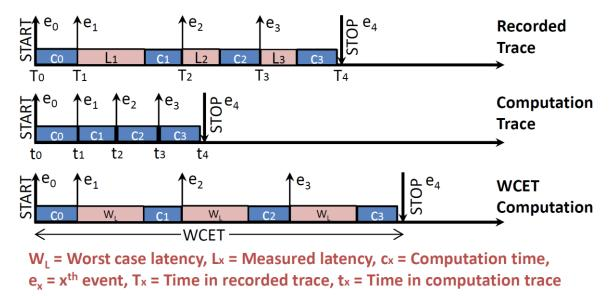
The computation trace can be considered constant if we start from the same cache, pipeline state and use the same input data.
