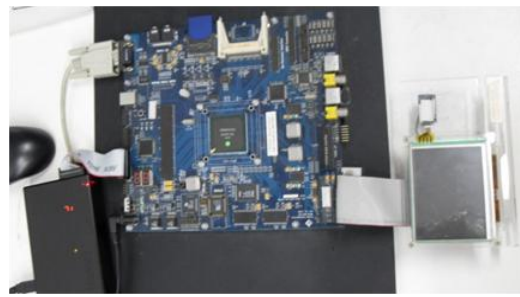
An H.264 Video Decoder implemented by the proposed technology
