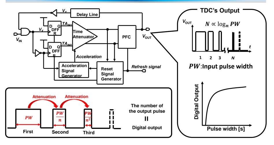
The time-attenuation-based TDC has the logarithmic input output characteristic. This circuit attenuates a input pulse width with a certain gain. This repetitive operation with a constant attenuation ratio (gain of less than unity) enables a logarithmic input–output characteristic.
