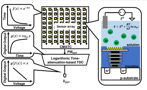
This work is the first to present a biosensor array that uses a newly-proposed bio-oriented logarithmic TDC.
