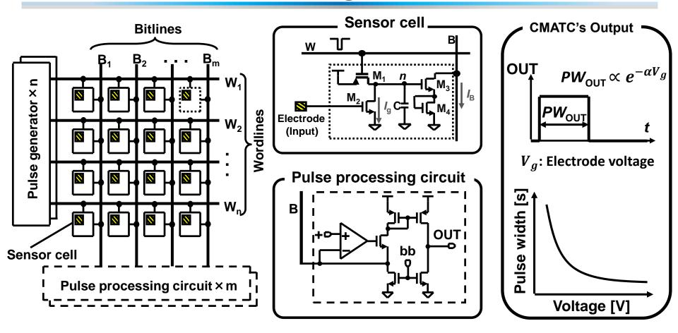
The CMATC consists of the pulse generator, sensor cell, and pulse processing circuit (PPC). The sensor cell outputs the current pulse, and the PPC converts the current pulse to the voltage pulse. The CMATC's output is as follows
