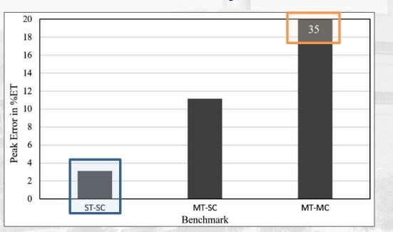
3% peak error for single-tasked application executing on single processor core (ST-SC)
