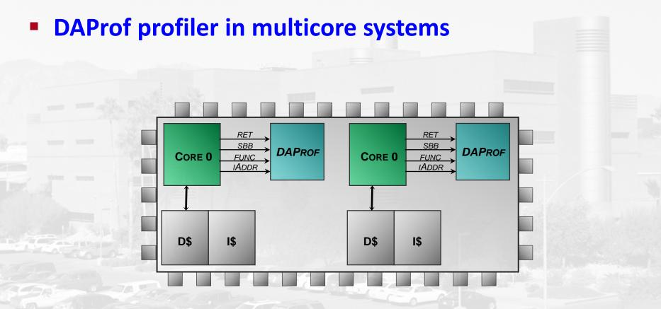
Direct application of DAProf to individual processor cores can lead to inaccurate <u>system</u> profile
