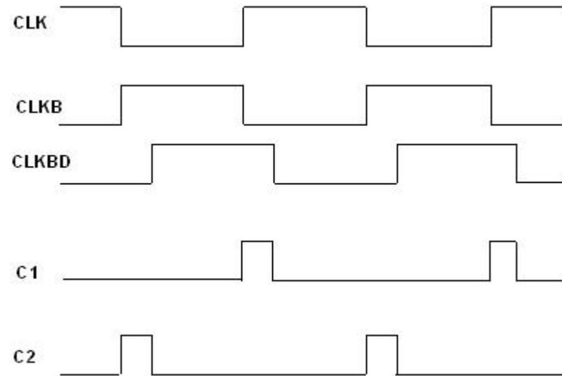
Figure 5. The timing diagram of C1 and C2 in DFFF.
