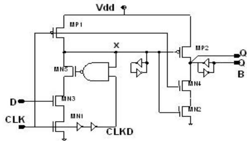
Figure 2. Circuit diagram of Sdff.
