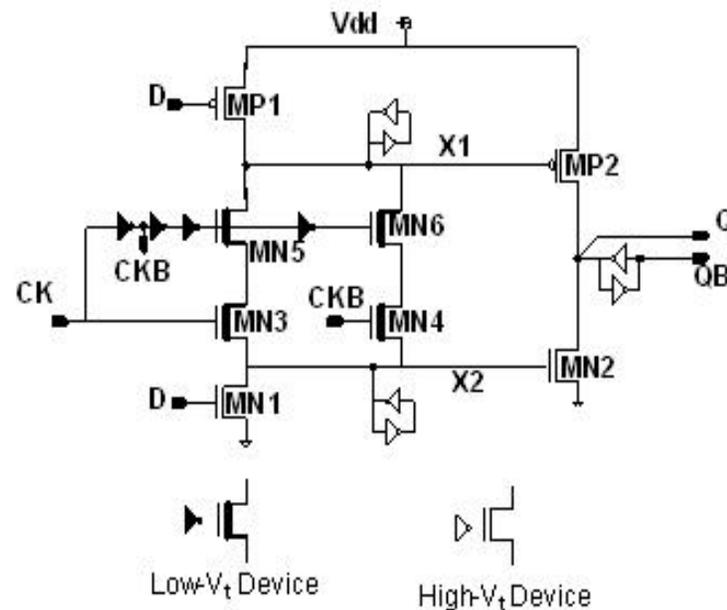
Figure 3. Circuit diagram of LSDFF.
