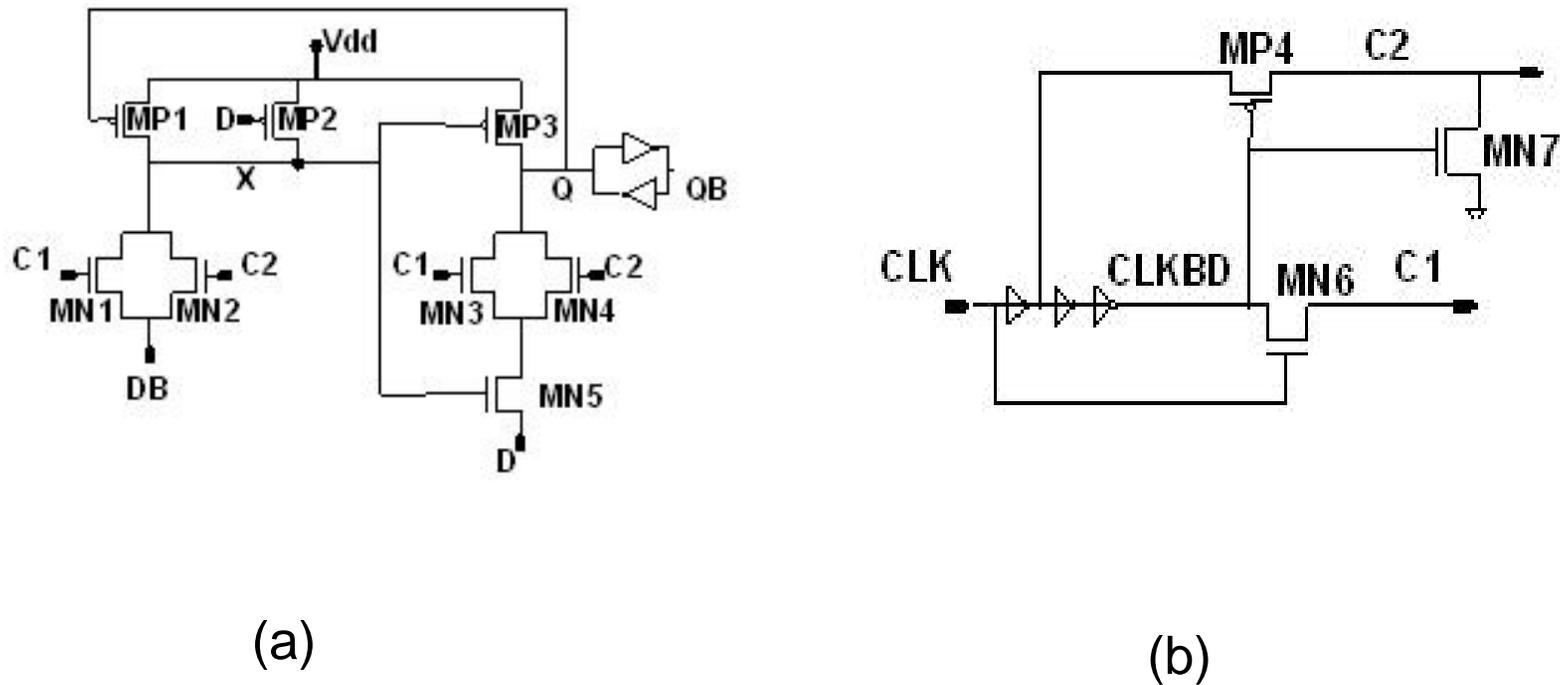
Figure 4. structure of (a) DFFF (b) clock-tree.
