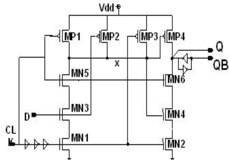
Figure 1. Circuit diagram of HLFF.
