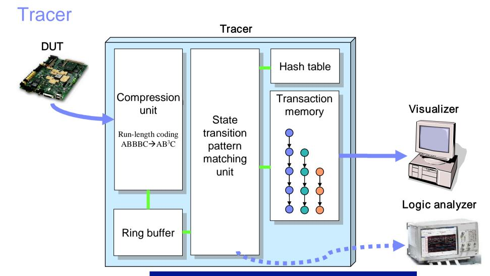
Generate a trigger when a new transition is detected. Rare transitions often give a good hit for debugging. They are often unexpected or not verified.
