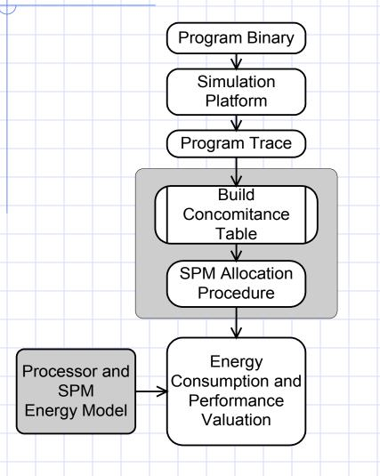
Concomitance table is build to provide information on the ranking of different basic block. SPM allocation procedure is to identify points in the program to insert the copy instruction.
