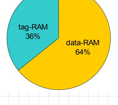
CACTI energy estimation tools shows that 36% of direct-mapped cache access energy is due to tag-RAM access. (0.18 µm)
