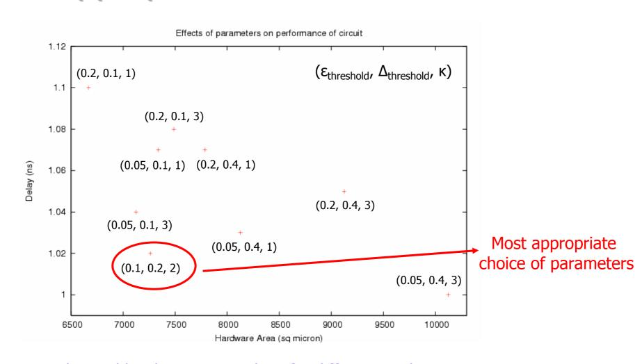
Delay and hardware area values for different implementations of a 8 x 8-bit multiplier generated by Selective Expansion for different values of  $\epsilon_{threshold}$ ,  $\Delta_{threshold}$ ,  $\kappa$ .
