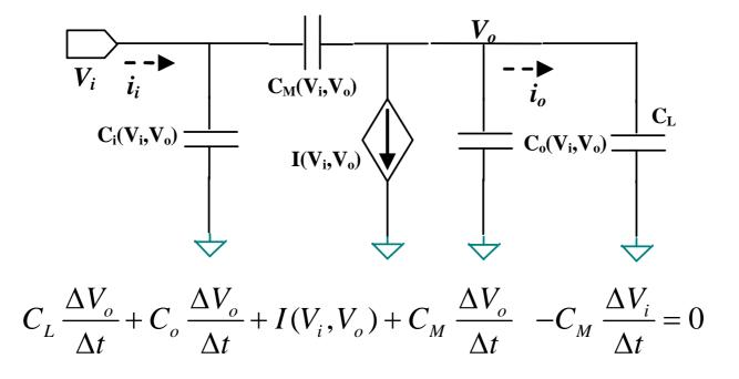
$V_o(t_{k+1})$ : Calculated based on  $V_o(t_k)$  and  $V_i(t_k)$ ,  $V_i(t_{k+1})$  and the current source and parasitic capacitance values
