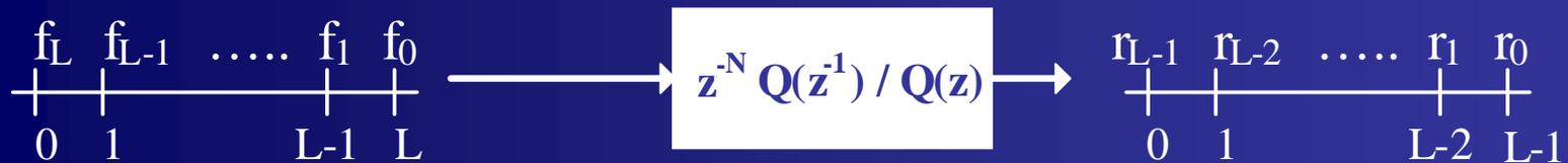
\*Find  $Q(z)$  such that energy output of the all-pass filter  $A(z) = z^{-N} Q(z^{-1}) / Q(z)$  is concentrated in time  $\geq L$ ,
