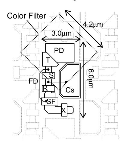
Rectangle Pixel Structure: High Area Efficiency Large Size PD: High Sensitivity
