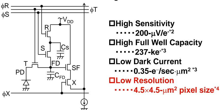
Pixel scaling is a very hard challenge because of the additional components switch S and Cs
