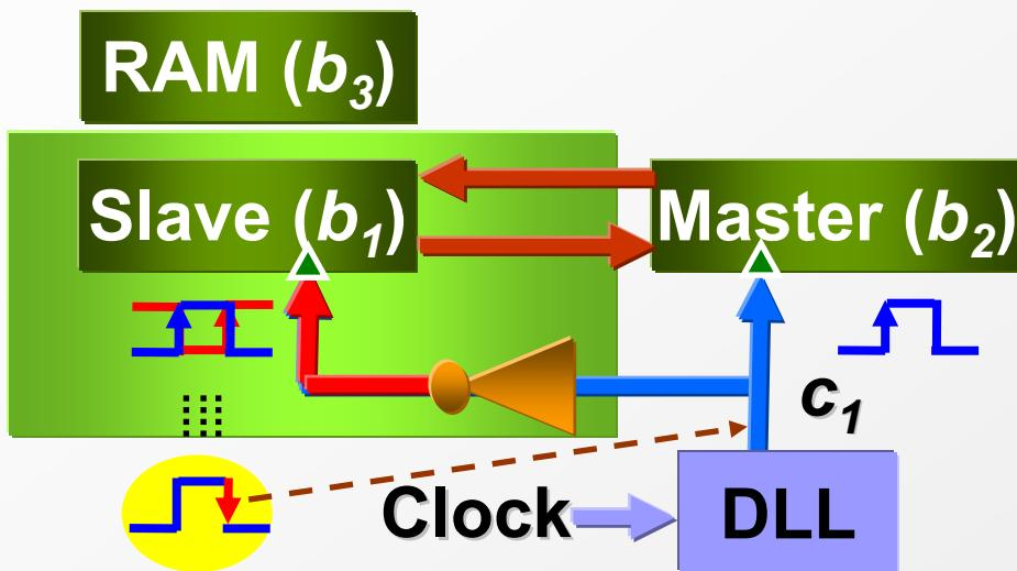
*The triggering edge of b<sub>1</sub>'s clock for c<sub>1</sub> must be fixed to be **positive**  $\leftrightarrow f_c(b_1, c_1) = 1$*
