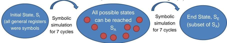
Symbolic simulation for 14 cycles is enough to ensure the correctness of customized design
