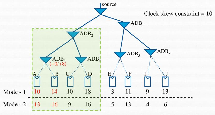
We have to retain ADB<sub>3</sub> (Case 1 at power mode 2) We can remove ADB<sub>4</sub> (Case 2 for all power modes)
