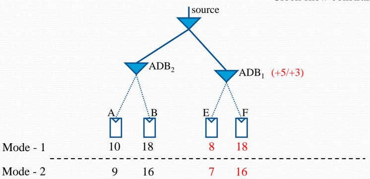
We have to retain ADB<sub>1</sub> (Case 1 at power mode 1 and 2) We can remove ADB<sub>2</sub> (Case 2 for all power modes)
