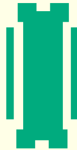
Sub-Resolution Assist Feature (SRAF)
