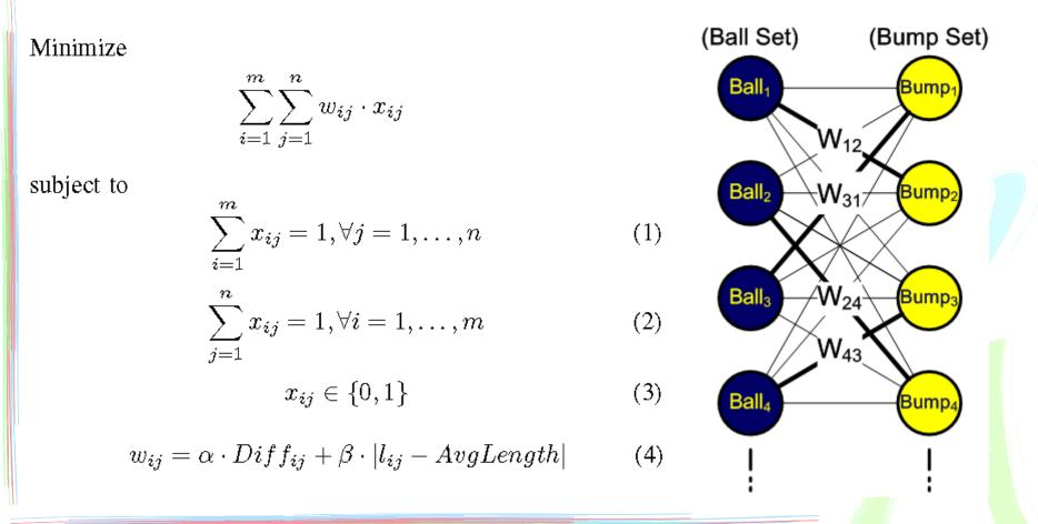
\* where  $Diff_{ij} = /Order_{ball_i}$ -Order\_ $bump_j$  is obtained through directly subtracting the order of  $Bump_j$  from  $Ball_i$ , and 2011/01/28 therefore calculating the upper bound of crossing number [14].
