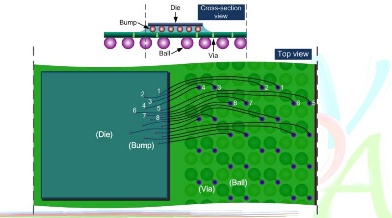
\*The monotonic routing is a route with no U-turn path. It consumes less routing resource and results in higher routing 2011/01/28 completion compared with nonmonotonic routing [6].
