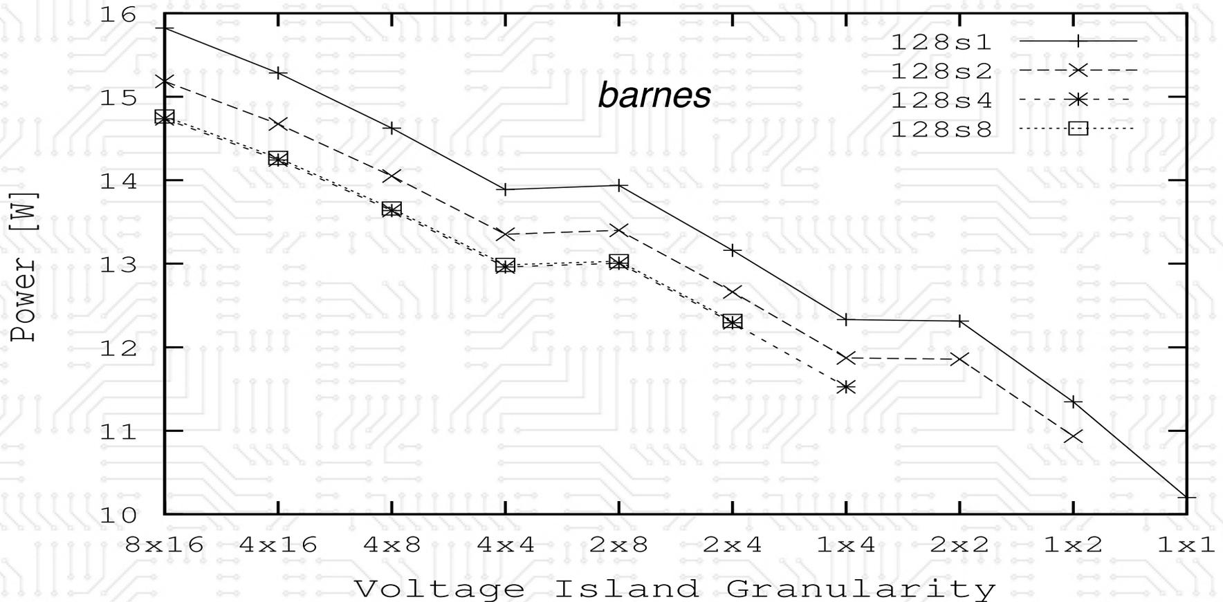
*the finer the granularity of the voltage island the higher the power savings.*
