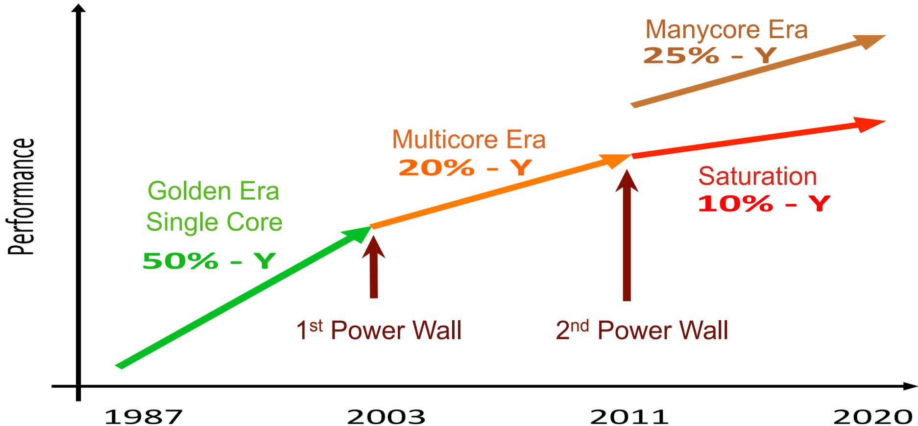
**Utilization Wall:** The percentage of a chip that can switch at full frequency drops exponentially due to power constraints.
