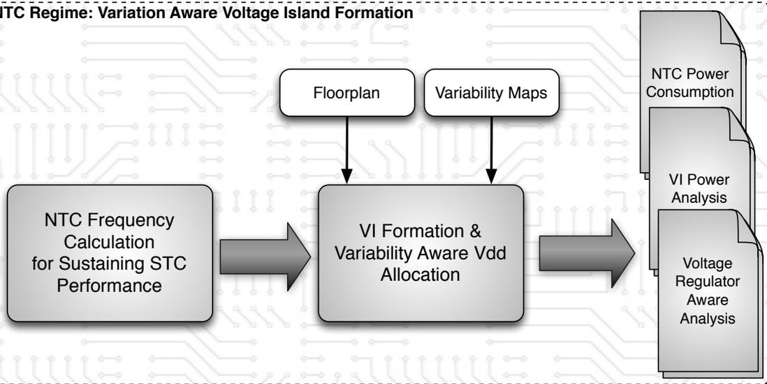
$$f_{NTC} = \frac{LC_{max}}{L_{min}} \times f_{STC}$$
