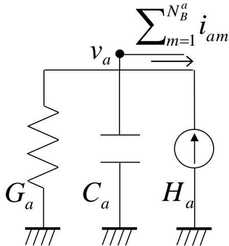
$$C_a \frac{dv_a}{dt} + Gv_a - H_a = -\sum_{b=1}^{N_B^a} i_{ab} \quad (1)$$
