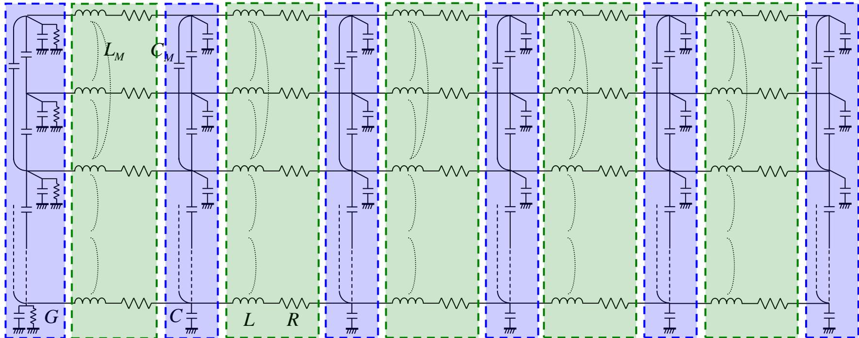
The equivalent circuit model of the entire MTL
