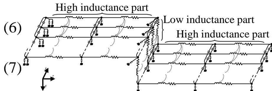
The maximum time step size used in HIE-block LIM **depends only** on the reactive elements in **the high inductance parts**
