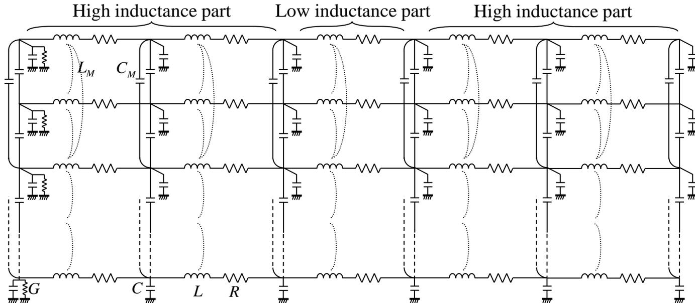
The equivalent circuit model of the entire MTL
