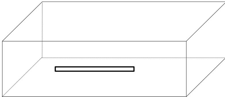
Geometry of the cavity-backed slot
