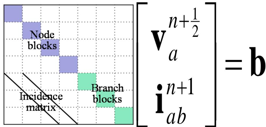
The coefficient matrix structure of unknown voltages and currents
