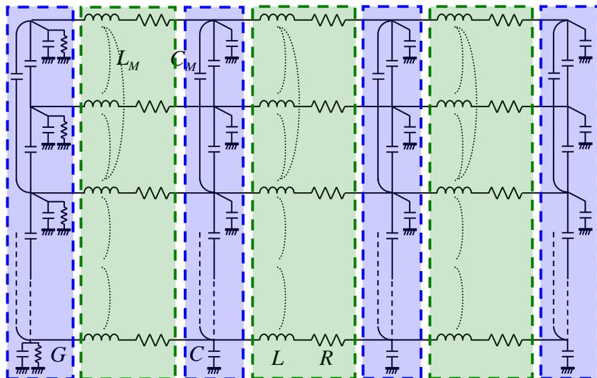
The structure of the coefficient matrix of unknown voltages and currents
