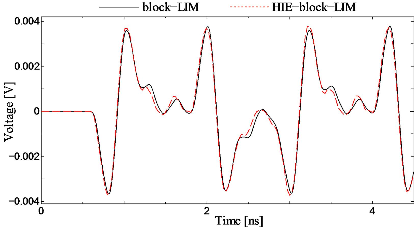
Waveform results of the node voltage
