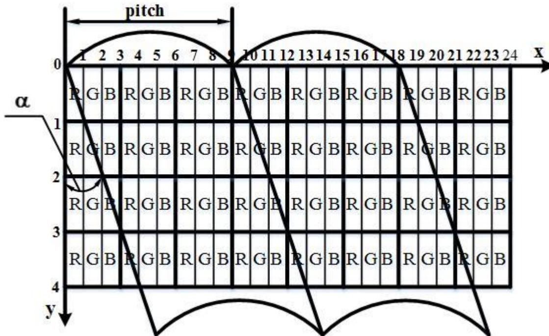
$$N(x, y) = \frac{(x - x_{\text{off}} - 3y \times \tan \alpha) \% \text{pitch}}{\text{pitch}} \times N_{\text{tot}} \quad (1)$$
