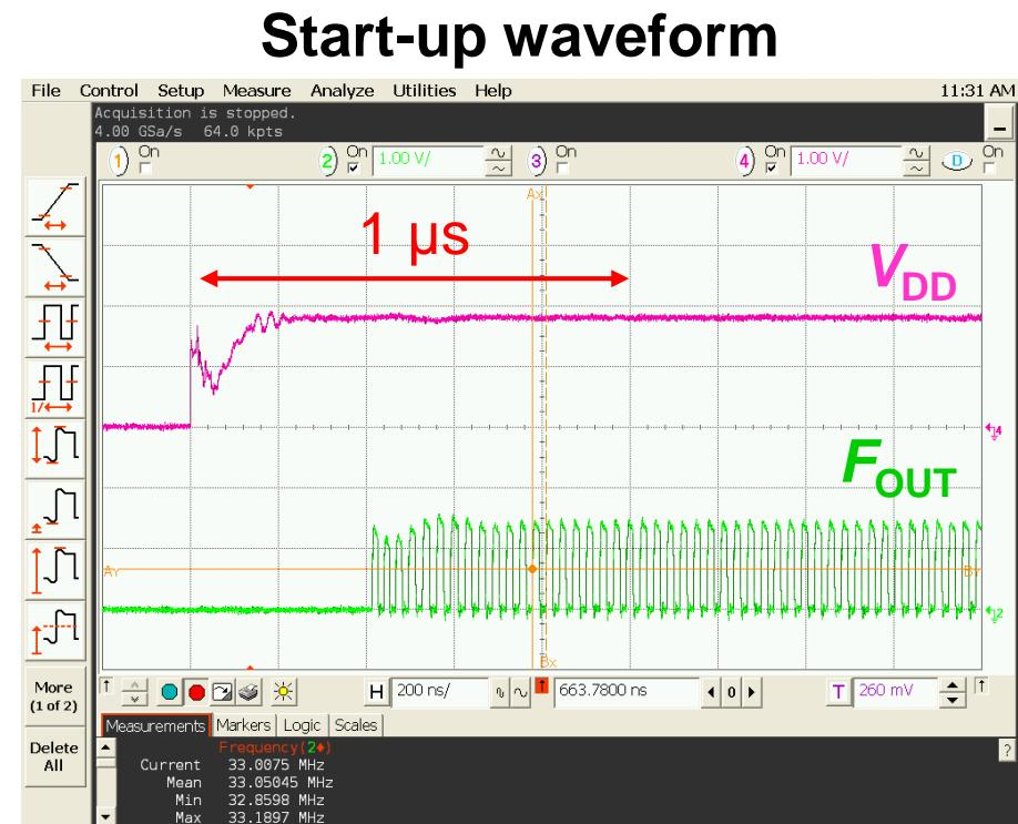
**Fast start-up, sub-1- $\mu\text{s}$ , with 32.6 MHz, 300.6  $\mu\text{W}$**
