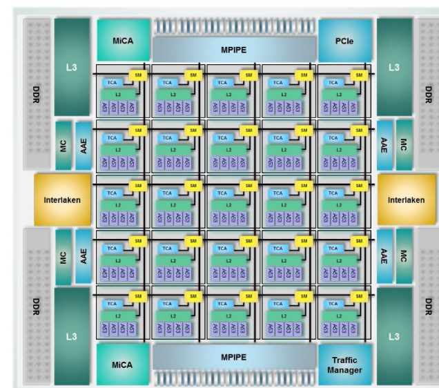
Ezchip MX-100: 5x5 mesh (4 core/Tile)
