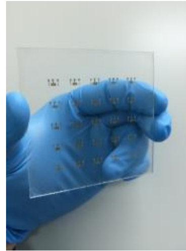
The structure and photo of fabricated SAM OTFT
