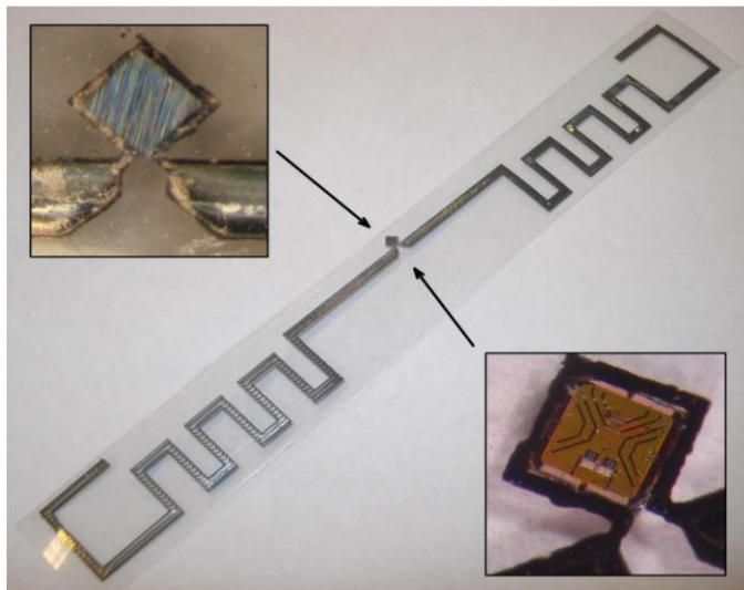
The UHF bonding-less module [3]
