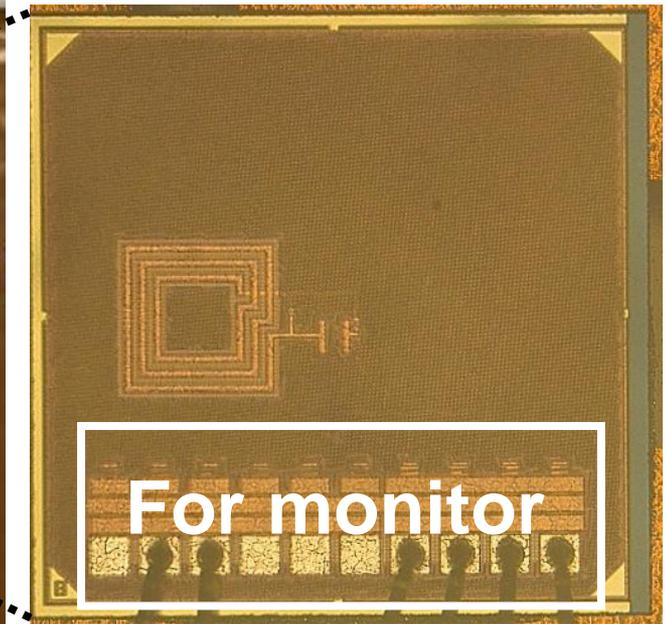
Photograph of proposed RFID module
