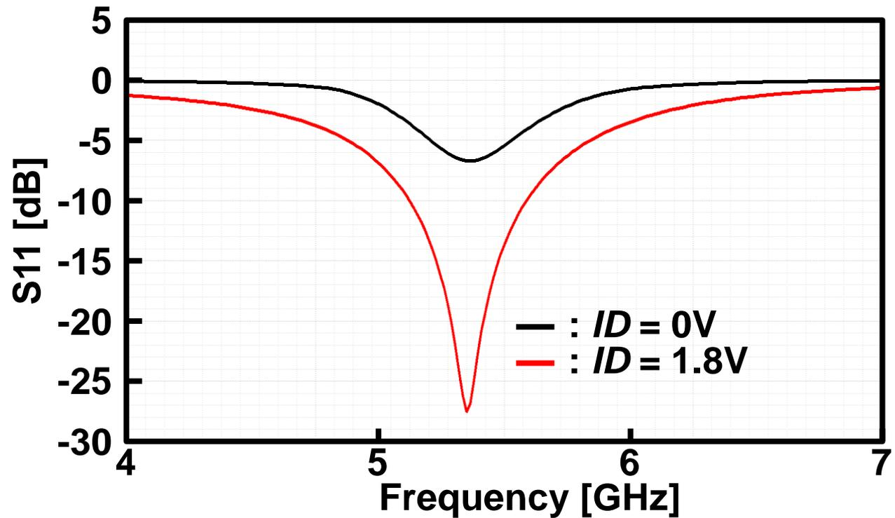
Reflection characteristics of antenna and internal circuit
