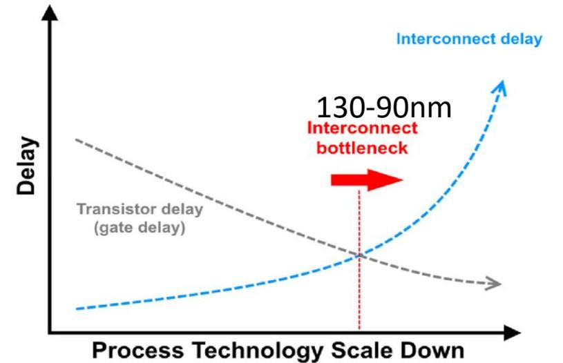
The impact of interconnect parasitic on overall circuit delay [1] and [2]
