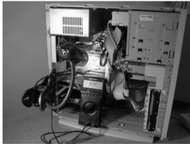
Figure 3. Experimental setup to induce memory errors, showing a PC built from surplus components, clip-on gooseneck lamp, 50-watt spotlight bulb, and digital thermometer. Not shown is the variable AC power supply for the lamp.
