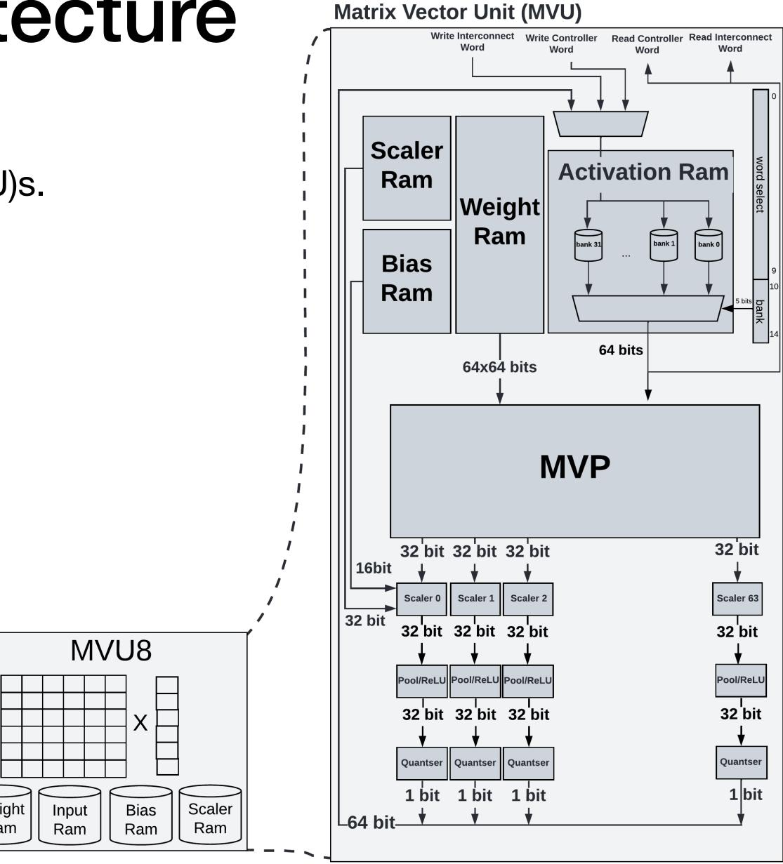
BARVINN: Arbitrary Precision DNN Accelerator Controlled by a RISC-V CPU
