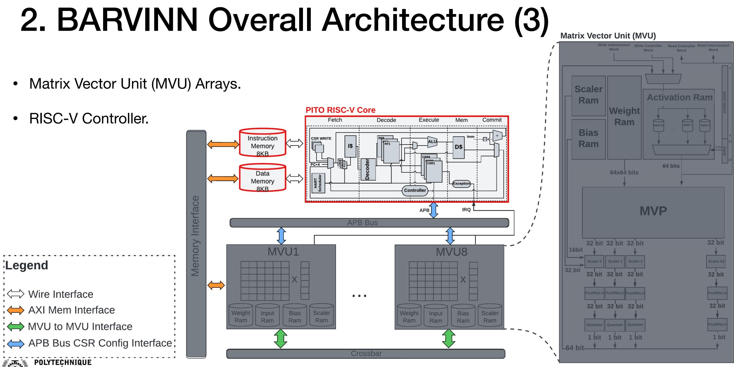
BARVINN: Arbitrary Precision DNN Accelerator Controlled by a RISC-V CPU
