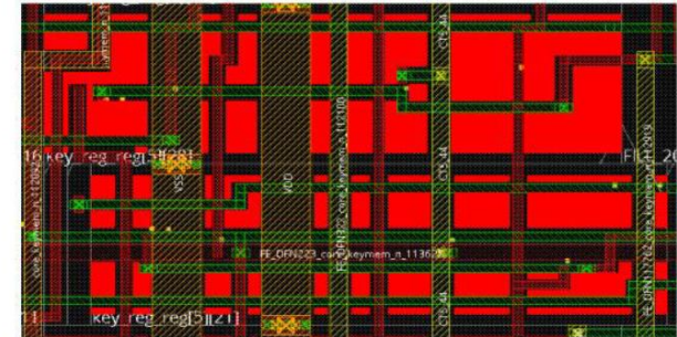
Security cells and nets exposed at frontside
