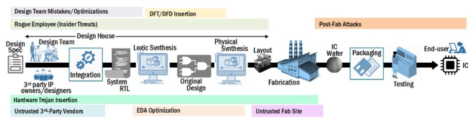
Potential sources of security vulnerabilities in modern SoC design flow
