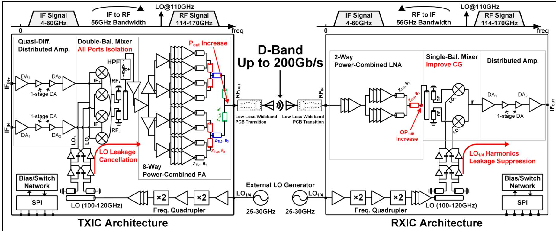
Heterodyne Architecture Front-End RF TX/RX Chipset.
