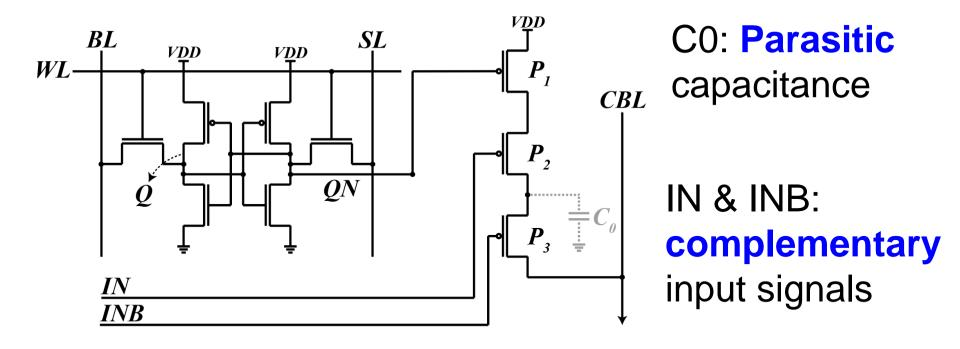
$\Delta Q = (VDD - V_{THP_3}) \times C_0$
