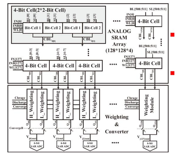
High precision weighting scheme Minimize power consumption and area overhead
