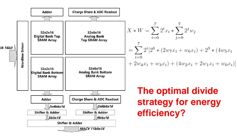
A Charge-Digital Hybrid Compute-In-Memory Macro with full precision 8-bit Multiply-Accumulation for Edge Computing Devices
