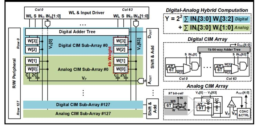
A 28nm 157TOPS/W 446.9Kb/mm2 Compute-In-Memory SRAM Macro with Analog-Digital Hybrid Computing for Deep Neural Network Inference
