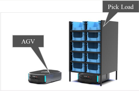
Figure 1:An AGV used in large logistics warehouses[7]
