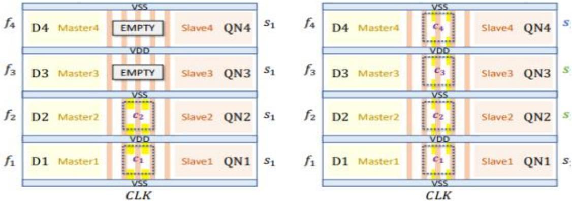
(c) Layout of MBFF in (a)      (d) Layout of MBFF in (b)
